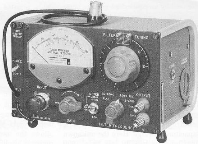
Figure 1. Type 1232-P2 Pre-amplifier attached to the 1232-A Tuned Amplifier and Null Detector
