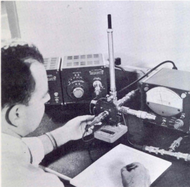
New uhf bridge in use measuring SWR of termination, with 7.5-cm reference air line connected as impedance standard.
