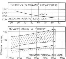
THE EXACT VALUE OF REFLECTOR VOLTAGE, PRODUCING MAXIMUM OUTPUT AT A CERTAIN FREQUENCY, VARIES FROM TUBE TO TUBE.
