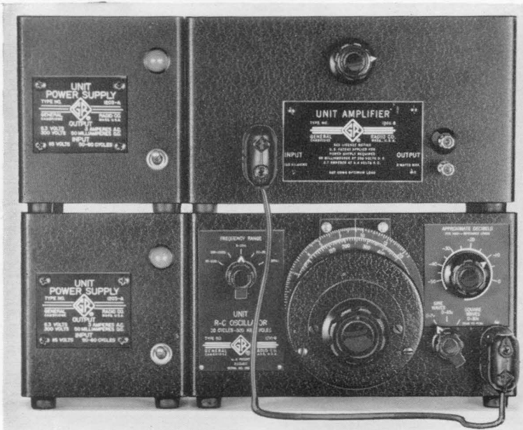
Figure 4. Panel view of Type 1210-B Unit R-C Oscillator and Type 1206-B Unit Amplifier with Type 1203-A Unit Power Supplies. The combination of these instruments delivers up to 3 watts of power with good waveform.
