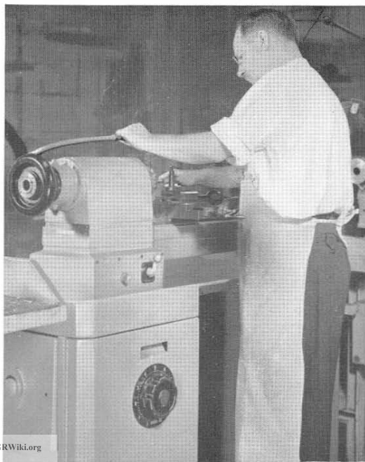
Figure 1. The new Type 1704-B Variac Speed Control installed on a bench lathe. The controller is installed just below the headstock where it is conveniently accessible, and the Variac, which is the speed adjustment control, is below the controller, on the bench cabinet. The chassis, which carries the transformers and rectifiers, is inside the cabinet.
