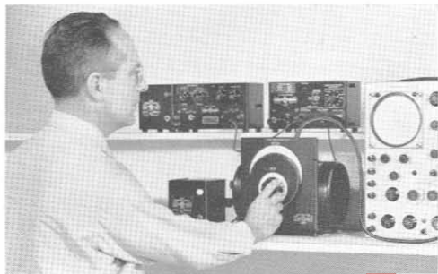
Figure 2. The Unit Pulser and Unit Pulse Amplifier, as set up to pulse a Type 1218-A Unit Oscillator at 1400 megacycles.
