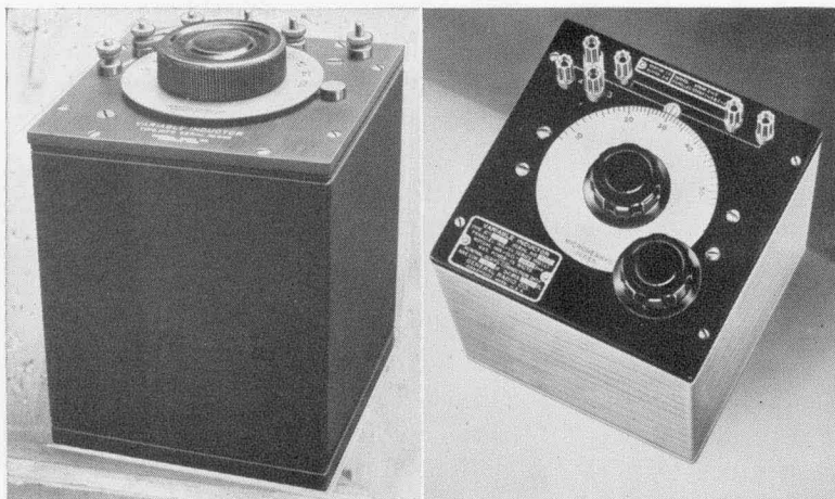
Since 1915, the radio-electronics industry has looked to General Radio for its laboratory standards. At the left is shown an early Type 107 Variable Inductor; at the right, today's direct-reading model.
