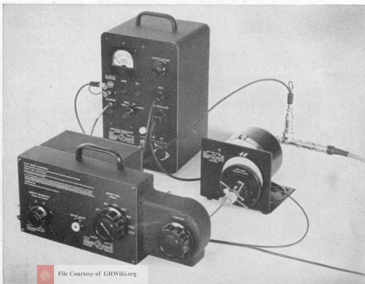
Figure 1. View of the new General Radio Sweep Drive and Amplitude-Regulating Power Supply set up to sweep a Type 1209-B Unit Oscillator.
