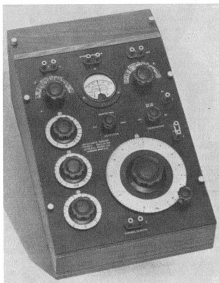
Figure 1. This front panel view of a Type 650-A impedance bridge shows its neat layout.
