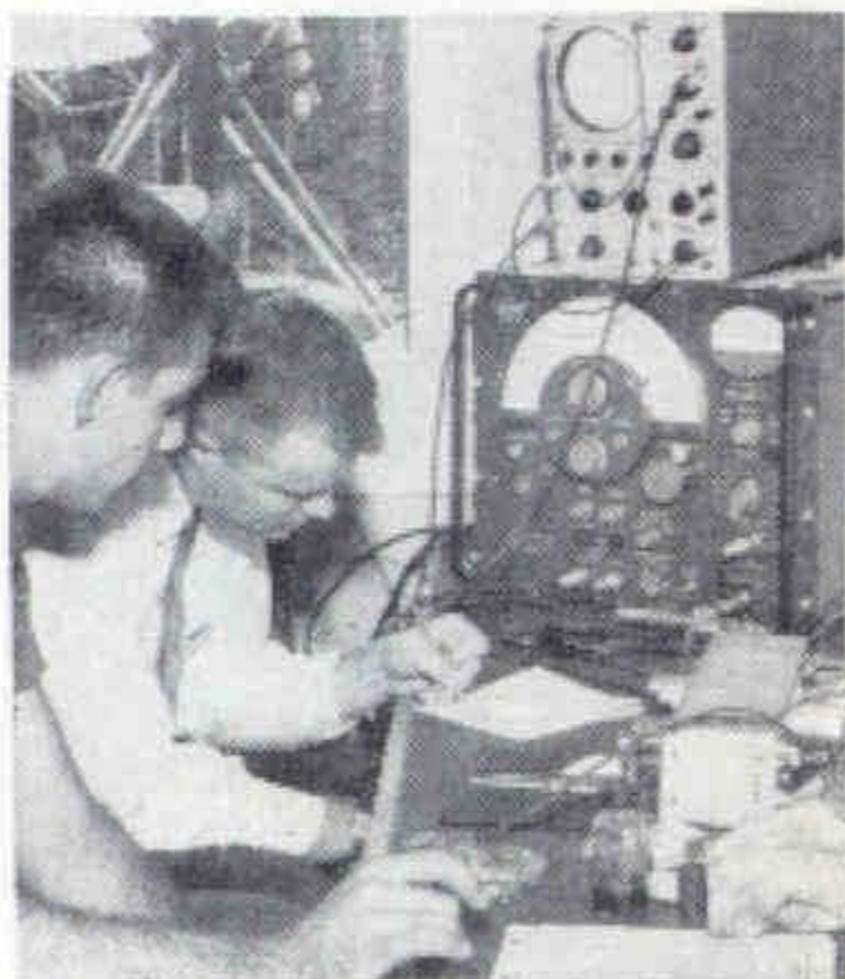
Engineers at Tapetone Electronics Laboratories, manufacturers of frequency converters for ham radio and for telemetry, are shown with the Type 1025-A Standard Sweep-Frequency Generator in aligning a converter. In this application, the stability and versatility of the generator save time and assure accurate alignment.
