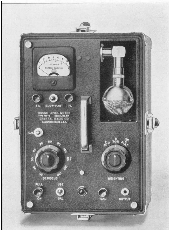
FIGURE 7. Panel View of the General Radio TYPE 759-B Sound-Level Meter.
