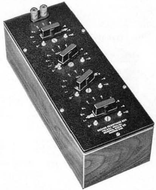
A TYPE 602-J Decade-Resistance Box, representative of a new line of boxes with submounted switches
