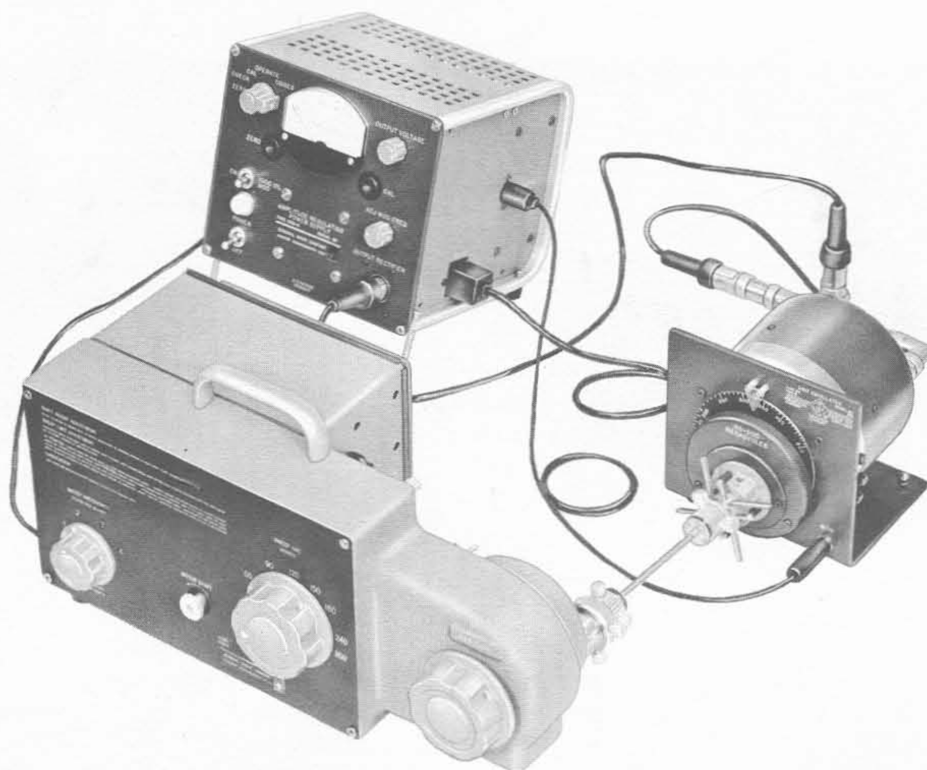
Figure 6. Type 1750-A Sweep Drive, Type 1263-B Amplitude-Regulating Power Supply, and Type 1208-B Unit Oscillator in Typical Setup.
