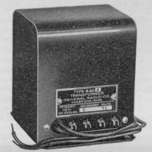
The alternating current tubes require a source of low voltage capable of delivering large current. The various types of tubes require several different voltages. The Type 440A transformer supplies voltages for all popular tubes and sufficient current for all ordinary receiver requirements. Filament supply is provided for filament, separate heater, power and rectifier tubes.
