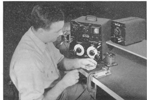
Figure 5. The Comparison Bridge used in adjusting an air-core inductor to 0.1% tolerance at General Radio's West Concord (Mass.) plant.
