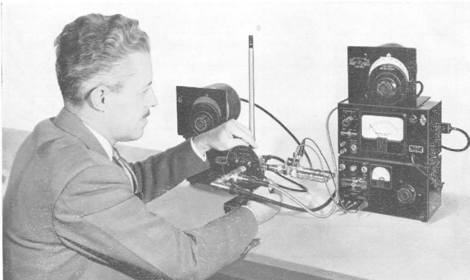
Figure 13. The Type DNT Detector Assembly is an excellent detector for use with the Type 1602-B U-H-F Admittance Meter, as shown here in a setup for measuring VSWR of a coaxial switch. The Type 1204-B Unit Variable Power Supply shown below the i-f amplifier is used to energize the solenoid in the coaxial switch.
