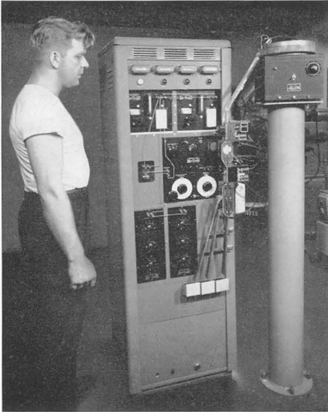
Figure 3. PROJECT TINKERTOY is the code name assigned to a program conceived and developed by the National Bureau of Standards for the Navy Bureau of Aeronautics, which involved the Modular Design of Electronics (MDE) and the Mechanized Production of Electronics (MPE).
