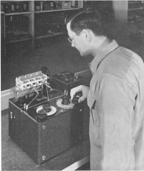
Figure 6. Another application in our own plant: testing and adjusting four-gang capacitors for proper tracking. The bridge is also used in the adjustment of ganged potentiometers.
