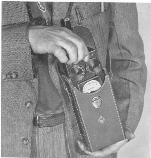
Figure 4. The Transistor Oscillator fits into the same convenient leather carrying case as the Sound-Survey Meter.
