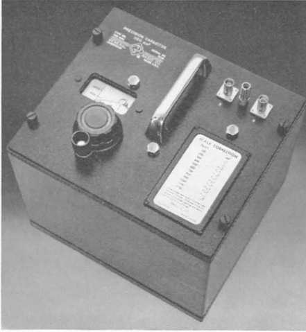
Figure 4. Panel view of a special Type 722 Precision Capacitor calibrated in direct capacitance. The coaxial terminals provide complete shielding for the leads.
