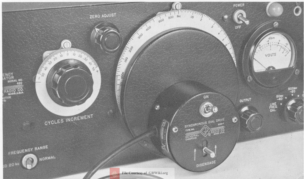
Figure 1. View of the Type 908-P2 Synchronous Dial Drive installed on a Type 1304-B Beat-Frequency Oscillator. The adjustable stops, which attach to the oscillator dial, are not shown.
