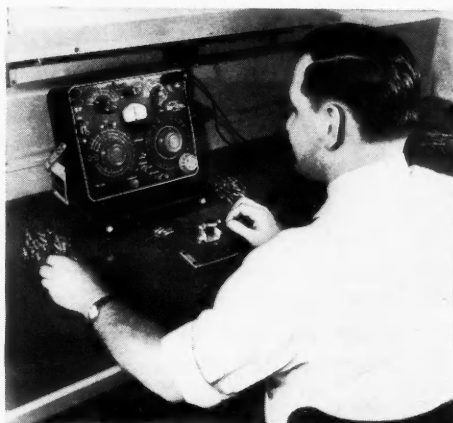
Figure 10. With the Test Jig, as shown here, the bridge can be set up for go-no-go testing to preset limits.
