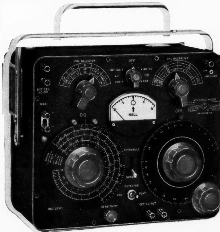
Figure 1. Panel view of the Type 1650-A Impedance Bridge. Note the many new features: Orthonull; built-in generator and detector; single D - Q dial; single pair of UNKNOWN terminals; bias terminals. For other external features, see cover.
