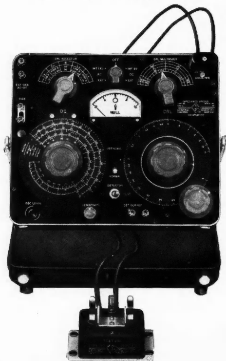
Figure 9. Bridge with Test Jig connected.
