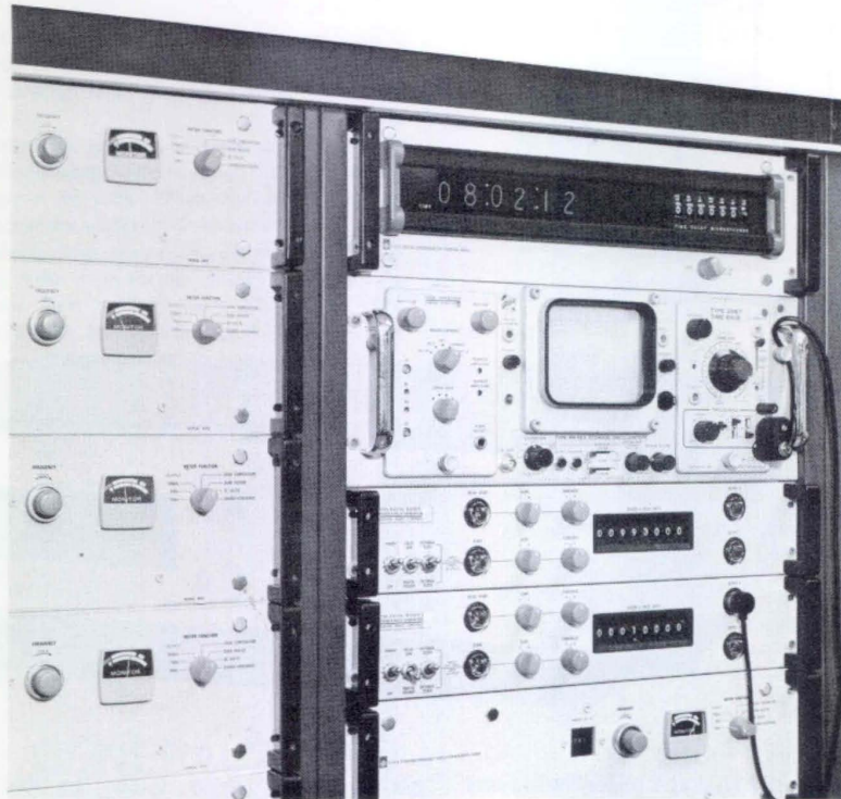
Figure 1. The 1399 and Loran C. An 1123 Synchronometer® digital time comparator, an 1124 Receiver, and two 1399's used to calibrate 1115-C Standard-Frequency Oscillators. The 1399's enable the system to derive time differences from a Loran system with arbitrary base rate.
