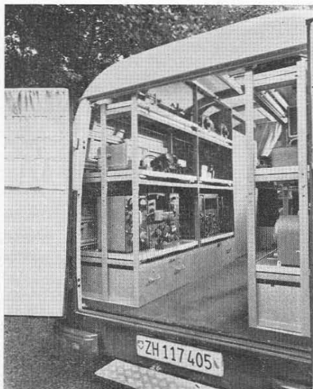
Interior of the station wagon, showing the tables securely installed for transporting.
