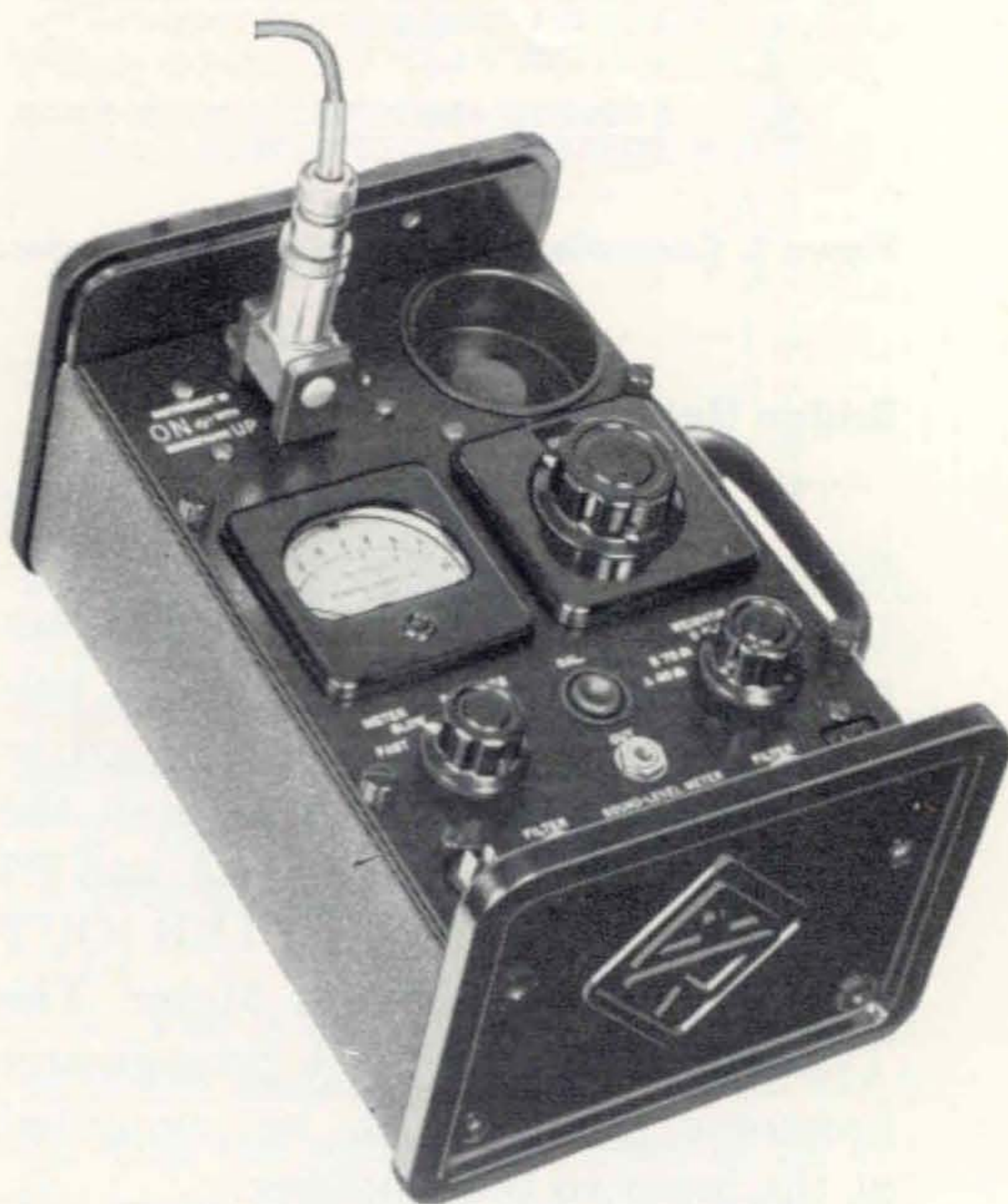
Figure 1. View of the Sound-Level Meter with microphone replaced by connector.
