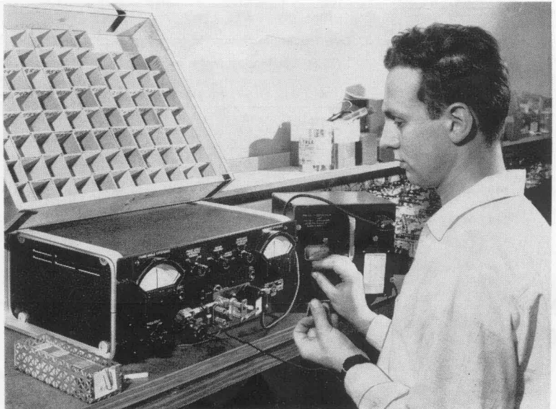
Figure 4. Mica for the Type 1409 Standard Capacitors is selected for low losses in this test setup using the Type 1605-A Impedance Comparator.
