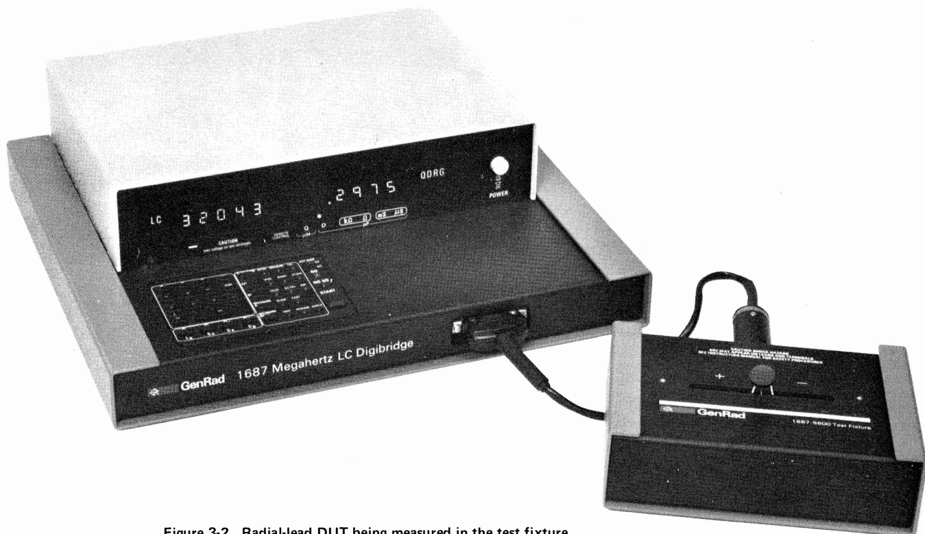
Figure 3-2. Radial-lead DUT being measured in the test fixture.
