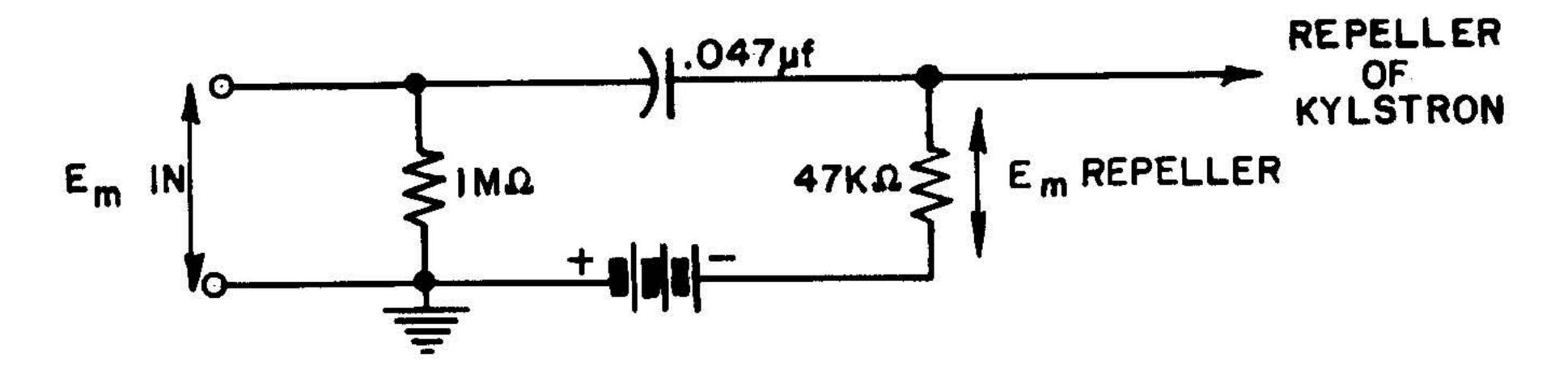
Figure 8. Coupling Circuit Between External Modulation and Repeller Voltage.
