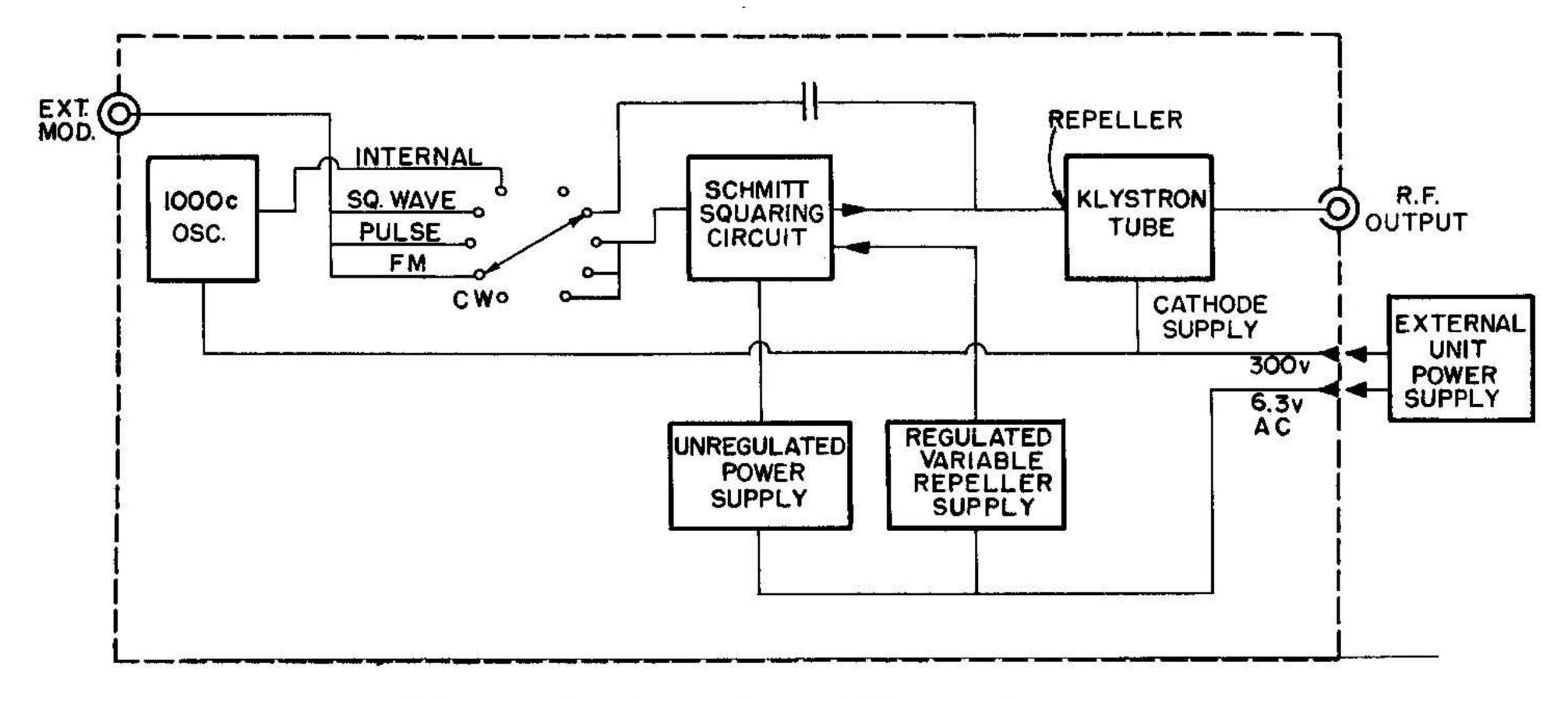
Figure 2. Functional Block Diagram.
