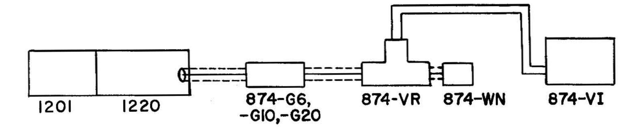
Figure 6. Recommended Detector Setup for Measuring Output. (Numbers are General Radio Instrument Type Numbers.)
