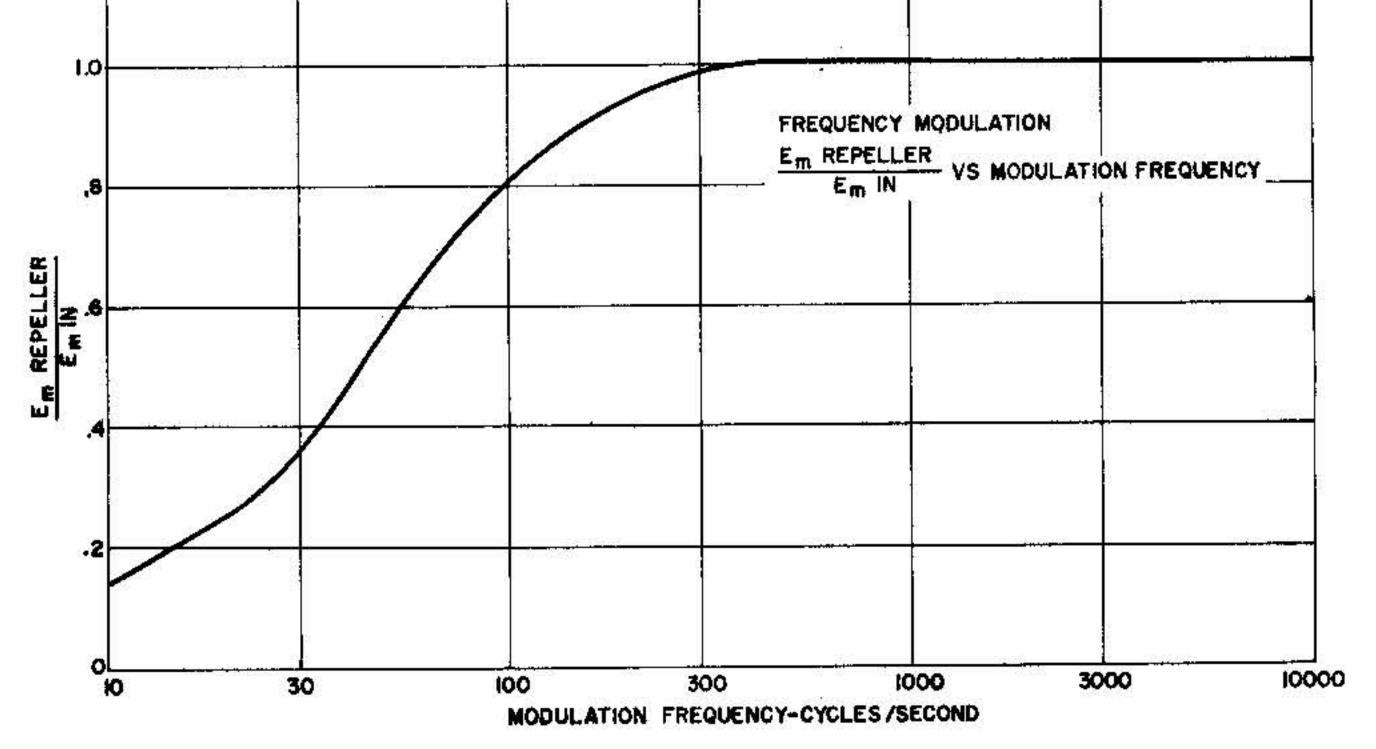
Figure 9. Ratio of Input to Repeller Voltage as a Function of Modulating Frequency.
