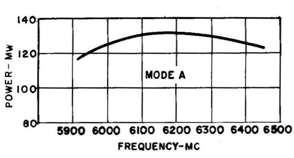
Figure 16d. Maximum Power Output vs Frequency.
