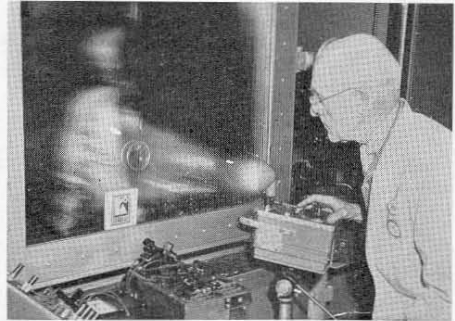
Figure 8. The Strobotac produces enough light to "stop" the motion of the fan through the eight layers of glass in the door of this altitude chamber. Some reflection is produced by the glass layers, but its effect is minimized by aiming the Strobotac flash into the chamber at an angle rather than head on. The new instrument's increased speed range now makes it possible to measure directly the speeds of fans operating at 400 cycles (24,000 rpm), which are commonly used in aircraft.
