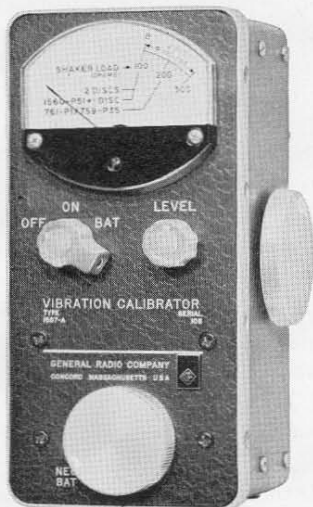
Figure 1. Panel view of the Vibration Calibrator.
