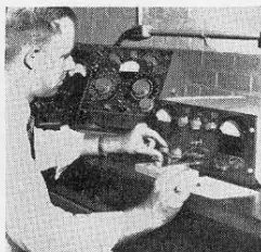
Measuring the collector-base capacitance of transistors with the Type 1605-A Impedance Comparator.
