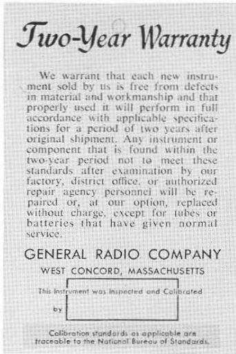
Figure 4. This 2-year warranty tag, which is supplied with all instruments, carries a statement of traceability.
