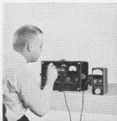
Calibrating the Type 761-A Vibration Meter with the Type 1557-A Vibration Calibrator.
