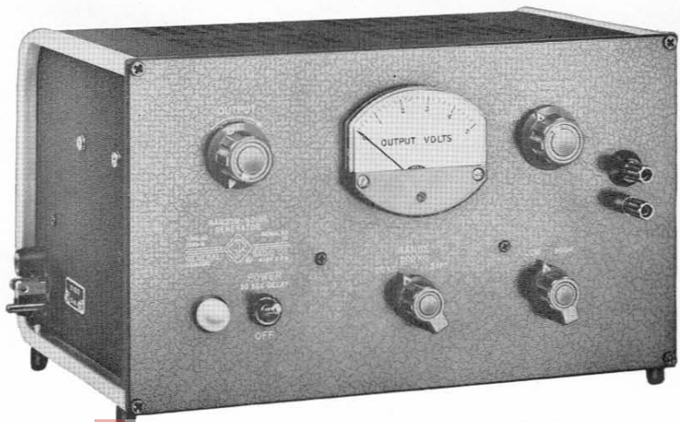
Figure 1. Panel view of the Type 1390-B Random-Noise Generator.
