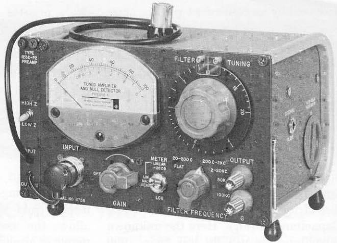
Figure 1. Type 1232-P2 Pre-amplifier attached to the 1232-A Tuned Amplifier and Null Detector
