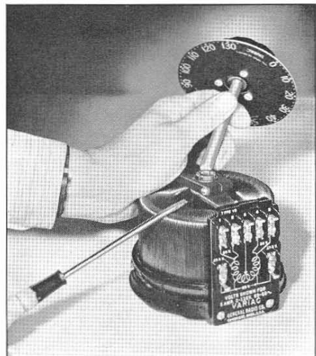
FIGURE 3. "A single screw loosens the shaft for removal or tightens it in assembly."
