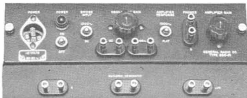
FIGURE 2. Panel view of the TYPE 650-P1 Oscillator-Amplifier, showing top of bridge panel. Connections are easily made from either the d-c or 1000-cycle terminals to the EXTERNAL GENERATOR terminals of the bridge.
