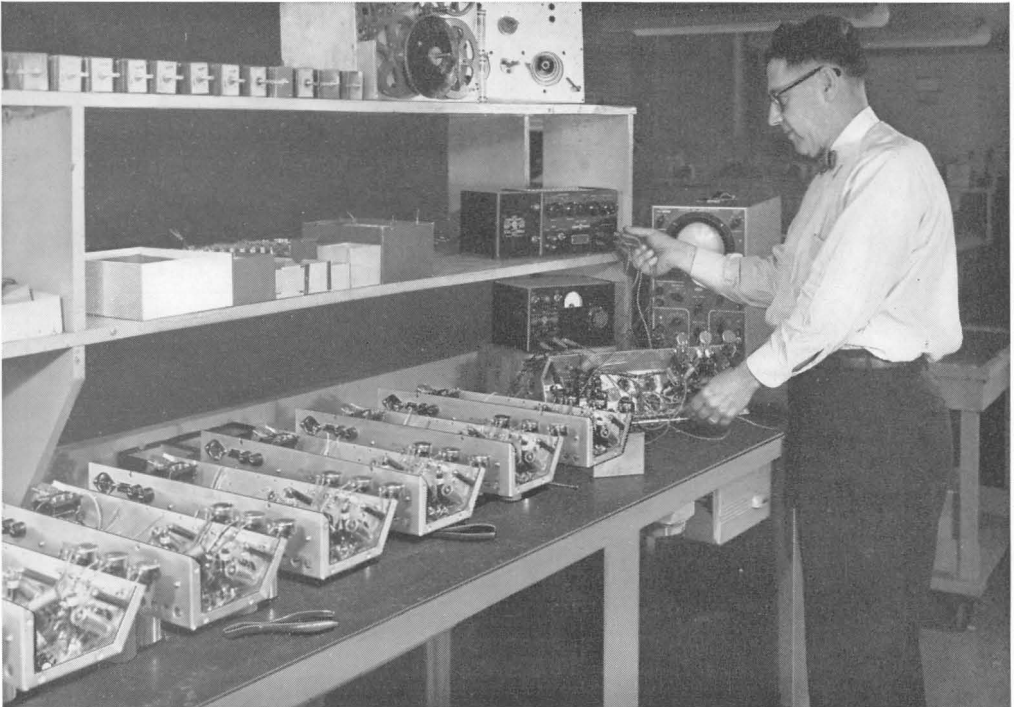
Figure 6. The Unit Pulser used for production tests on amplifier assemblies.
