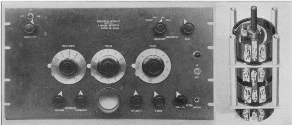
Figure 14. Panel view (left) of a Western Electric detector used in checking coils. The four-gang rheostat controlled by the TUNING dial is shown at the right.
