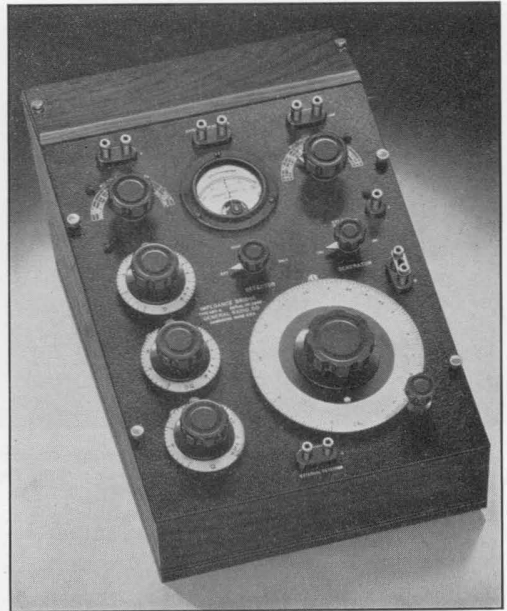
Figure 11. Panel view of the Type 650-A Impedance Bridge. The logarithmic rheostat controlled by the large dial was shown in Figure 2, Part I, of this article.
