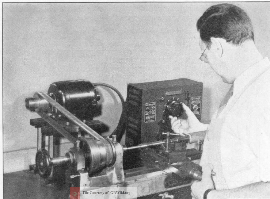
Figure 1. View of a Type 1700-A Variac Speed Control installed on a bench lathe.
