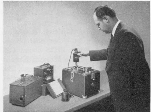
Figure 5. Calibrating a sound-level meter with the sound-level calibrator. A Type 723-B Oscillator and Type 727-A Vacuum-Tube Voltmeter provide the standard 400-cycle voltage.
