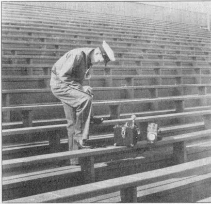
FIGURE 6. Showing the sound-level meter and oscillograph as used in measuring the over-all characteristic of the system.
