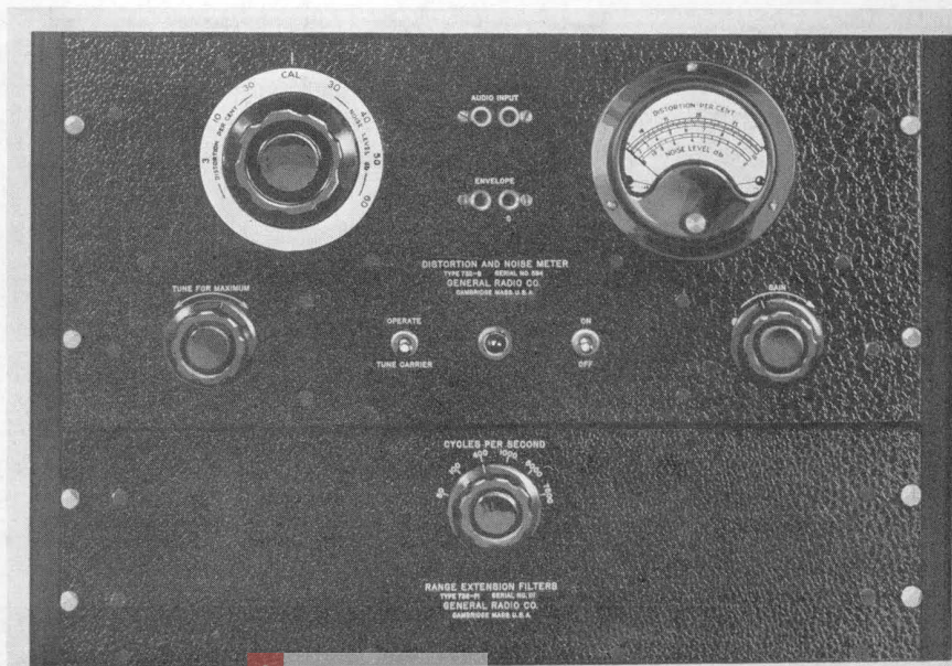
FIGURE 1. Panel view of TYPE 732-B Distortion and Noise Meter and TYPE 732-P1 Range-Extension Filters.
