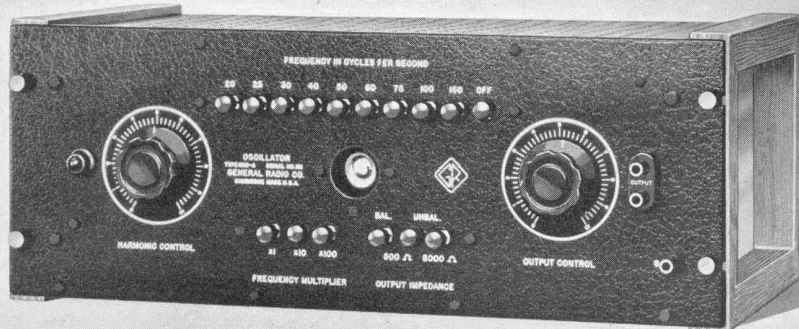
FIGURE 1. Panel view of the TYPE 608-A Oscillator. Both frequency and output impedance are selected by means of push-button switches.
