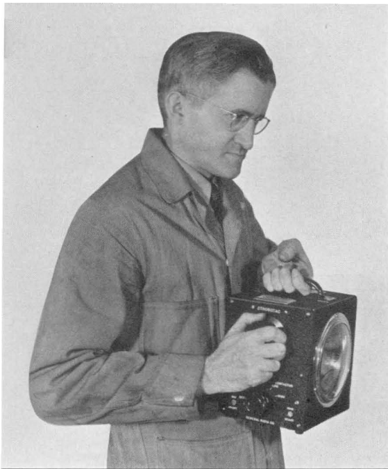
FIGURE 2. The controls and the scale of the Strobotac are arranged for maximum convenience. When the instrument is held in the left hand, as shown, the right hand is used to adjust the speed, which is read directly from the scale on the top of the case.
