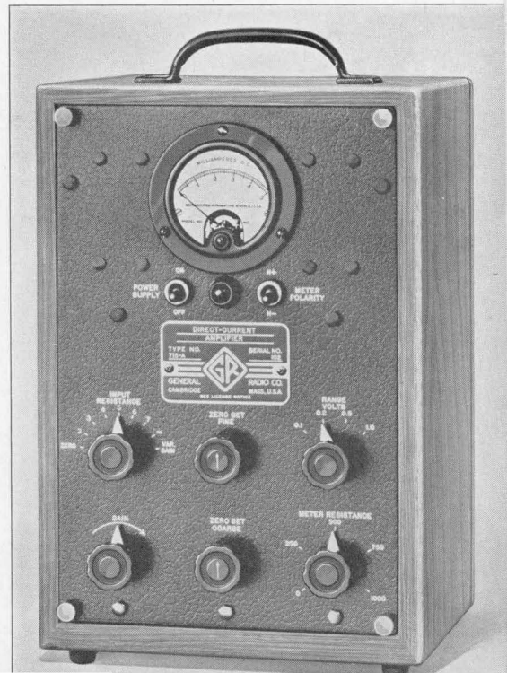
FIGURE 3. The TYPE 715-A Direct-Current Amplifier in walnut cabinet.
