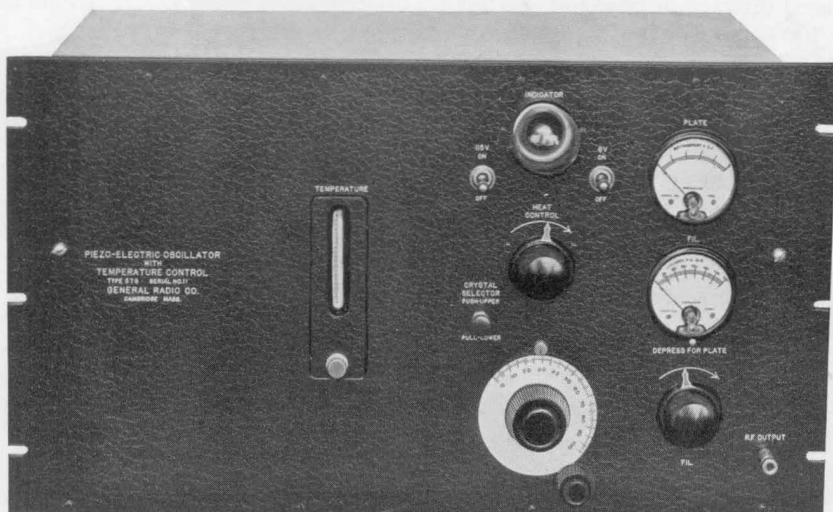
TYPE 575-A Piezo-Electric Oscillator with Temperature Control
