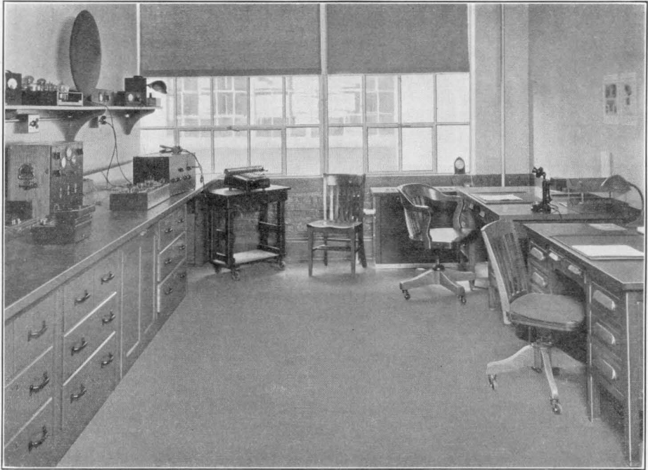
FIGURE 2. A typical laboratory. It will be noted that the power outlets are so located that they may be used conveniently for apparatus on the bench or on the shelf. Each outlet has its own switch and pilot lamp
