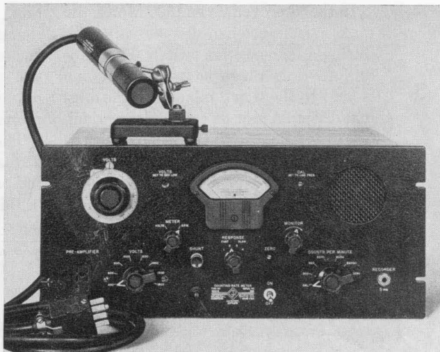
Figure 1. Panel view of Type 1500-B Counting-Rate Meter with counter tube and probe stand.
