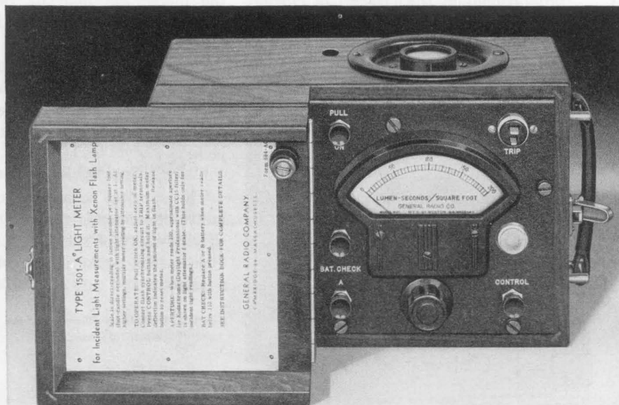
Figure 1. Panel view of the Light Meter, showing meter scale and controls.
