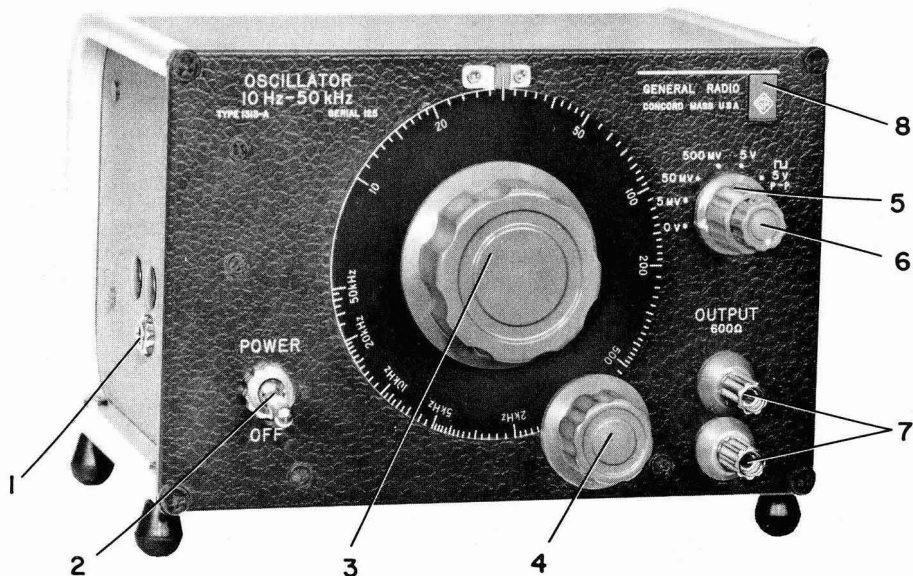
Figure 1-2. Controls and connectors on the Type 1313.
