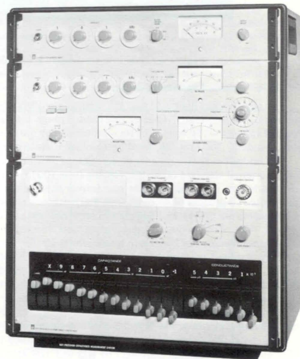
Figure 8. GR Precision Capacitance-Measurement System. Top to bottom: 1316 Oscillator, 1238 Detector, 1616 Precision Capacitance Bridge
